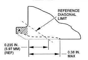
Any remaining Area 'A' lip material is sufficient to permit axial material removal up to 0.38 inch (0.97 mm) limit. Surface shall have a smooth contour and 0.020 inch (0.51 mm) minimum blend radius. Removal of all Area 'A' material is permitted when axial material removal is less than 0.235 inch (5.97 mm) diagonal limit. Surface shall have a smooth contour and 0.020 inch (0.51 mm) minimum blend radius.
