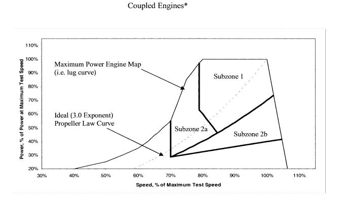
\*shown for engines capable of operating on the E3 Duty Cycle
