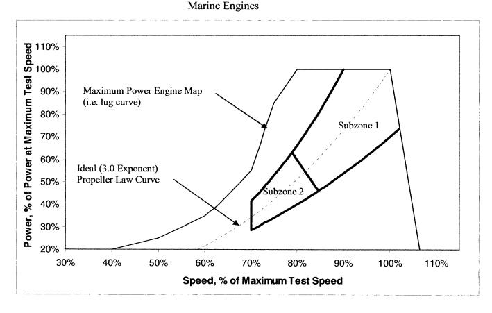
(c) Figure 2 of this Appendix illustrates the default NTE zone for recreational marine engines certified using the duty cycle specified in § 1042.505(b)(2), except for variable-speed marine engines used with controllable-pitch propellers or with electrically coupled propellers, as follows:
