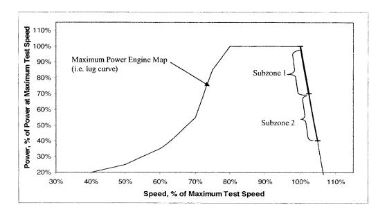
(f) Figure 5 of this Appendix illustrates the default NTE zone for variable-speed auxiliary marine engines certified using the duty cycle specified in § 1042.505(b)(5)(ii) or (iii), as follows:
