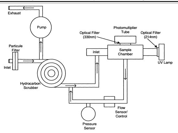
Figure 1. UVF SO<sub>2</sub> analyzer schematic diagram.
