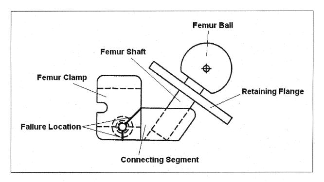
Figure 1: Illustration of femur assembly
