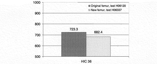
Figure 5: HIC 36 values for tests of the Britax Marathon child seat where the original femur failed (H06120) and for a new femur which did not fail (H06337).
