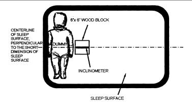
Figure 4D: Top View of CAMI Dummy and Inclinometer, Rotated 90°, Placed in the Sleep Surface for the Mattress Flatness Test
