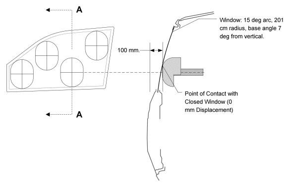
Figure 6 – NPRM Displacement Measurement at Target A2
