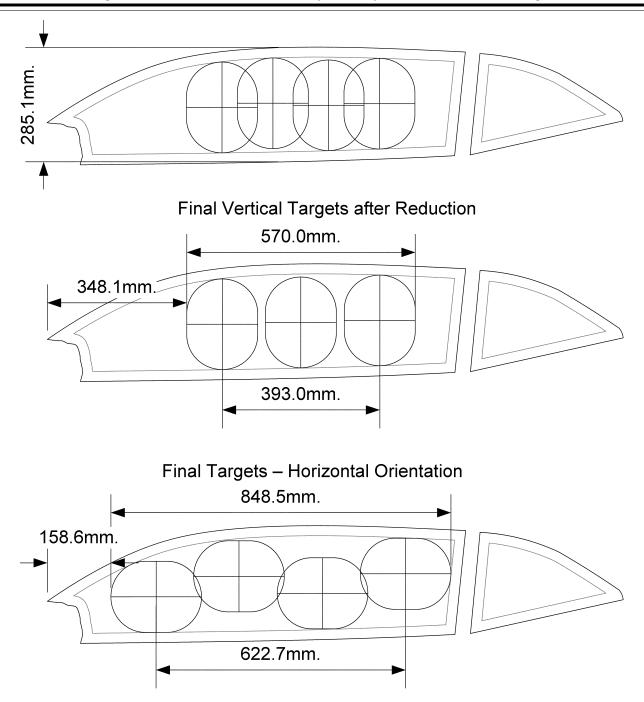
**Figure 15** – Side daylight opening of a MY 2010 Chevrolet Camaro (approximate dimensions), with the height of the window increased by 3% - Showing initial and final vertical targets and final horizontal targets.
