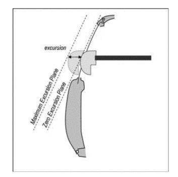
Figure 5 - Alliance Displacement Measurement Method.
