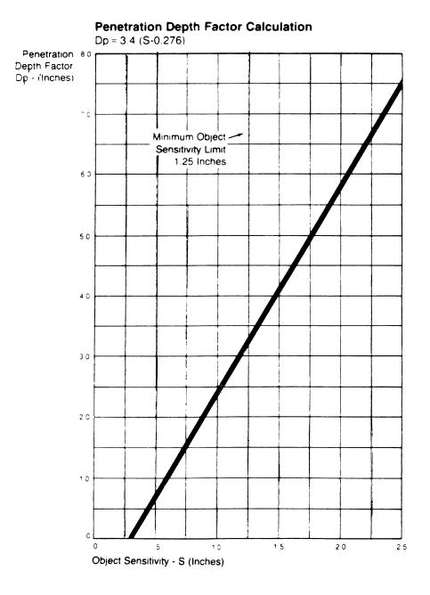
(vi) The presence sensing device location shall either be set at each tool change and set-up to provide at least the minimum safety distance, or fixed in location to provide a safety distance greater than or equal to the minimum safety distance for all tooling set-ups which are to be used on that press.
