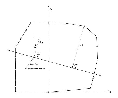
NOTE: LARGEST LIQUID HEIGHT ABOVE THE POINT WHERE THE PRESSURE IS DETERMINED = Z B
